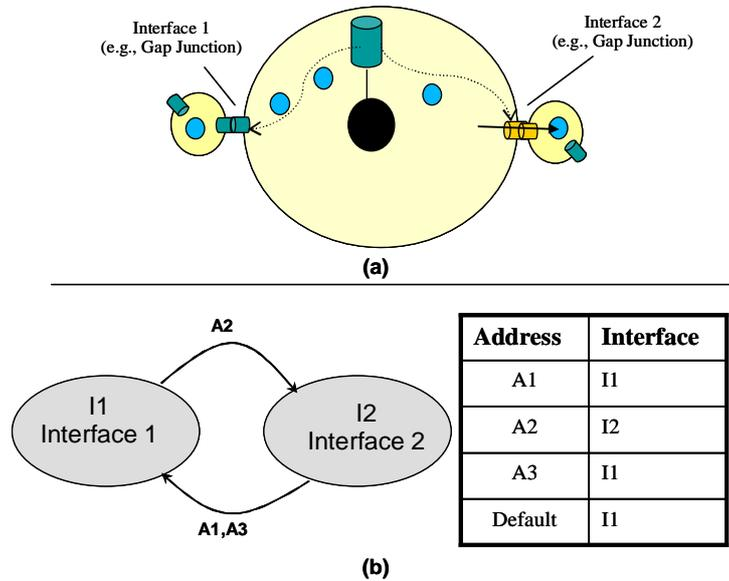
**Fig. 5.** (a) Schematic diagram of cell with two distinct molecular communication interfaces, (b) Address/Interface state diagram and switching table.
